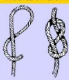
The figure of eight is a stopper knot, used to tie off the end of a line. It is commonly used to prevent the ends of the sheets of sails from pulling through blocks, eyebolts or fair-leads.
